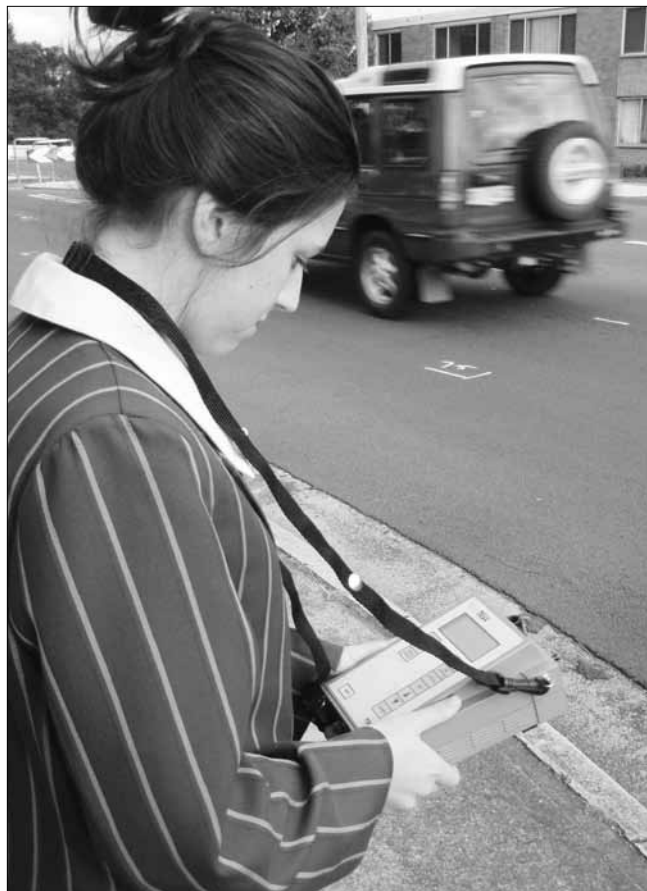
A student using a DustTrak to measure particles generated by traffic
