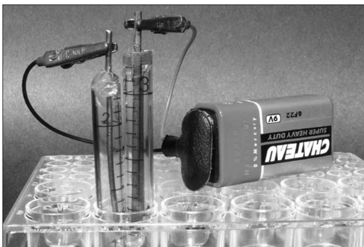
Easy setup demonstrates electrolysis using only 5 ml of solution.
